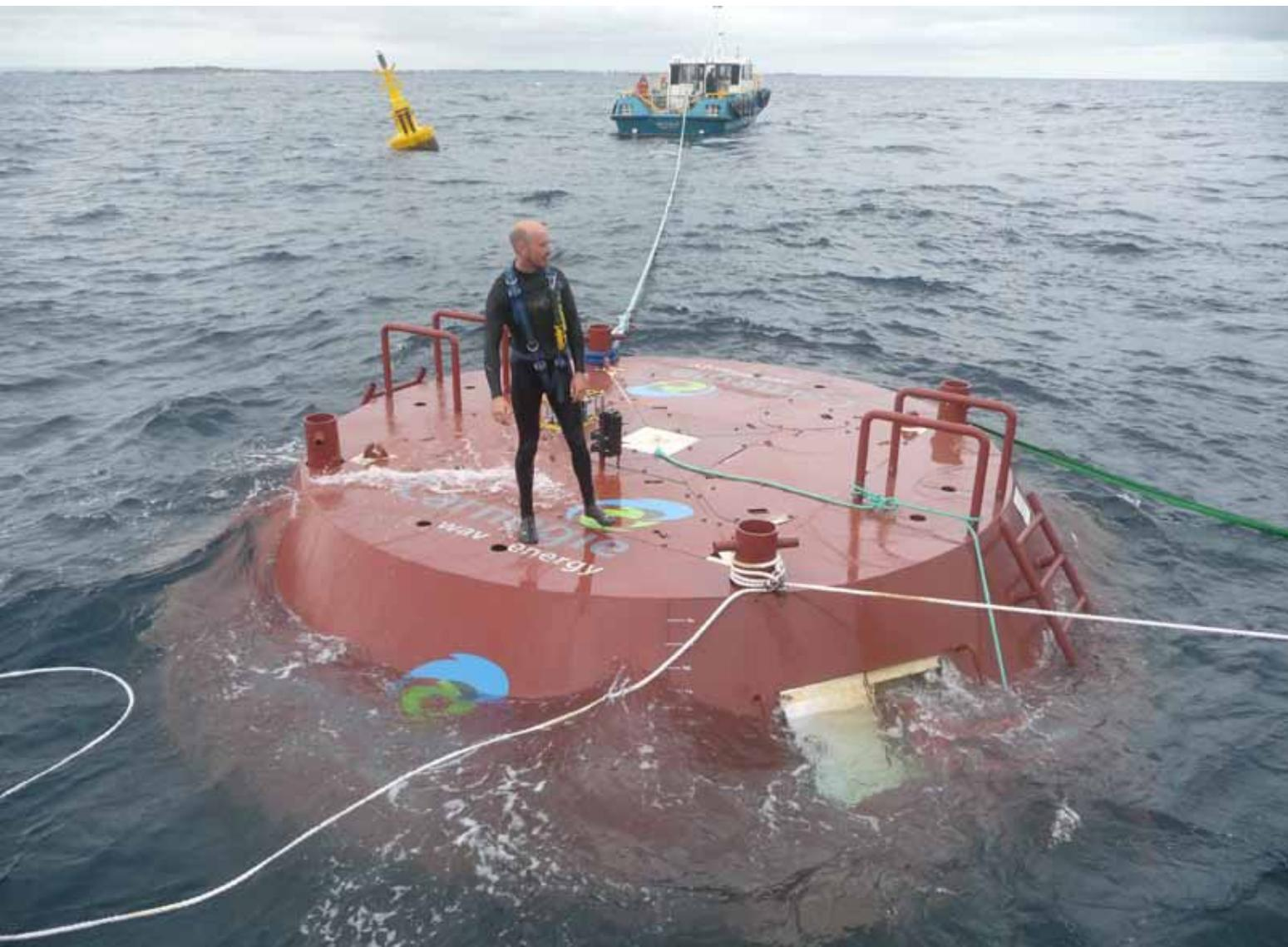
Investment in new low emissions technology – buoyant actuator for Carnegie Wave Energy's wave power demonstration plant. Photo – Carnegie Wave Energy
